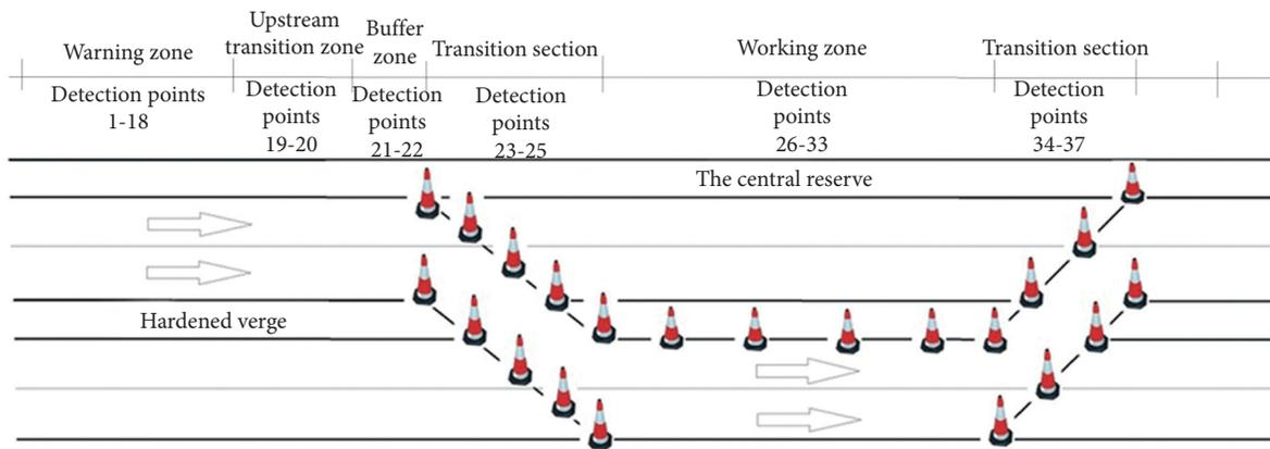
FIGURE 3: The layout of data detection points.
