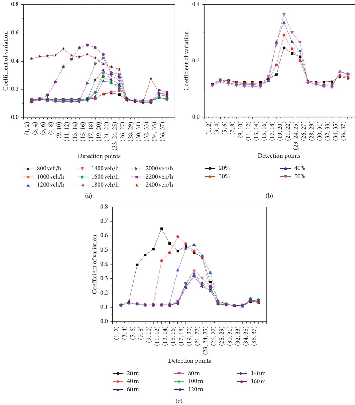
FIGURE 5: Coefficient of variation varies with each factor. (a) Coefficient of variation varies with traffic volume. (b) Coefficient of variation varies with the proportion of large vehicles. (c) Coefficient of variation varies with the length of the transition section.
