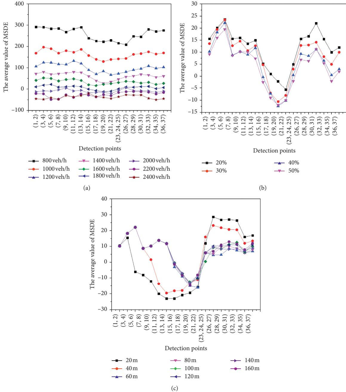
FIGURE 6: The minimum safe distance equivalent varies with each factor. (a) The average value of MSDE varies with traffic volume. (b) The value of MSDE varies with the proportion of large vehicles. (c) The average value of MSDE varies with the length of the transition section.
