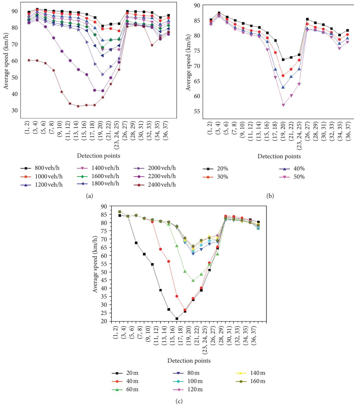
FIGURE 4: Average speed varies with each factor. (a) Average speed varies with traffic volume. (b) Average speed varies with the proportion of large vehicles. (c) Average speed varies with the length of the transition section.
