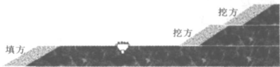
图 3 半填半挖段双侧路基加宽横断面图 Figure 3 transverse cross section of bilateral widening cut fill subgrade
