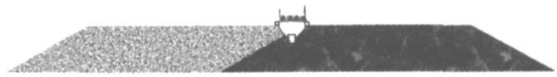
图 1 填方段单侧路基加宽横断面图 Figure 1 transverse cross section of one-sided widening fill embankment
