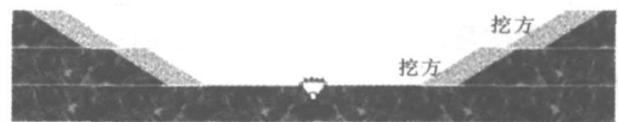
图 4 挖方段双侧路基加宽横断面图 Figure 4 transverse cross section of bilateral widening cut subgrade
